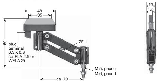
Lift  $\pm 10 \text{ mm}$ , swivel  $\pm 15 \text{ mm}$ , contact pressure: ca. 3 N
