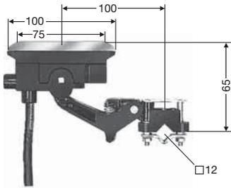
c/w 2 m cable · lift & swivel  $\pm 20$  mm
