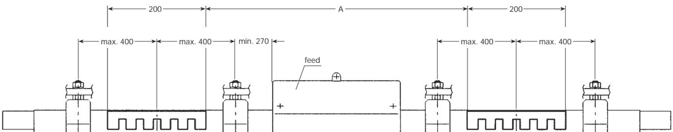
In order to avoid voltage bridging and for clearing of maintenance, control and live areas use two isolating sections.
