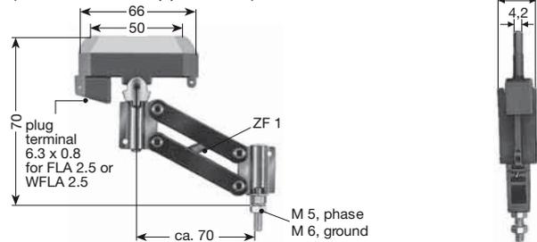
Lift  $\pm 10 \text{ mm}$ , swivel  $\pm 10 \text{ mm}$ , contact pressure: ca. 3.5 N
