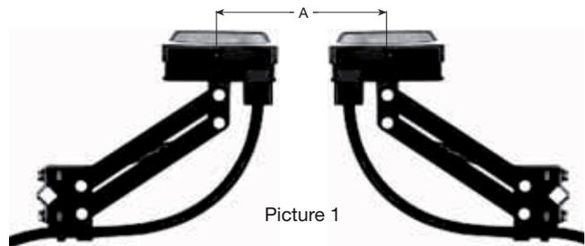
$A < 300 \text{ mm}$  conductor support spacing 0.8 m
