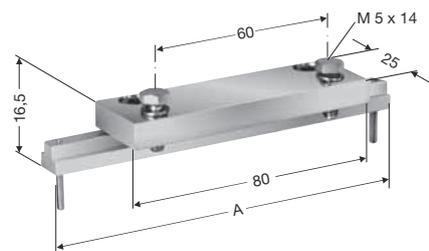
(Distance between conductor sliding surface and track = 24 mm; corresponds to compact hanger KA 15/6)
