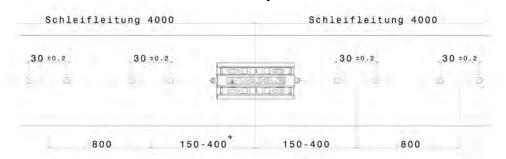
$<sup>^{\</sup>star}$  only applies if the connecting cap can be supported. For exposed connectors adhere to the spacing of 150 mm.
