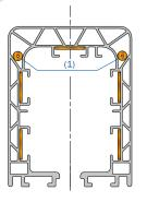
(1) The heating system consists of two cables arranged on either side.
