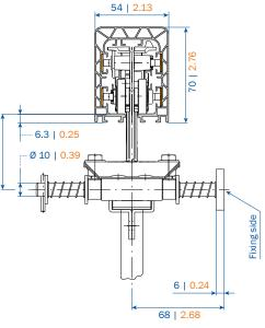
max. horizontal offset 10 mm (0.39 in)max. vertical offset 10 mm (0.39 in)
