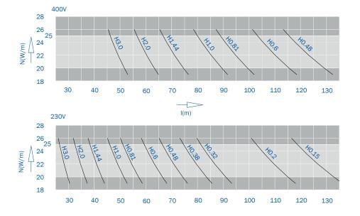
Heating capacity Watt/m: N' =  $\frac{U^2}{R \cdot L^2}$
