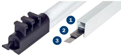
The code rail consists of the support profile <sup>(1)</sup>, the code strip <sup>(2)</sup> and the sliding strip <sup>(3)</sup>. The sliding strip serves for the mounting and sliding guidance of the APOS LKG-17 reading head.
