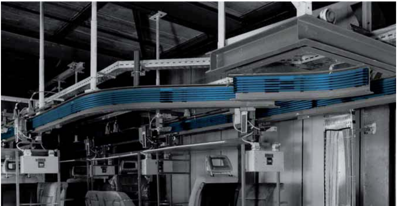
New material handling techniques (automated overhead monorails) require reliable electrification and use U 15 conductors.
